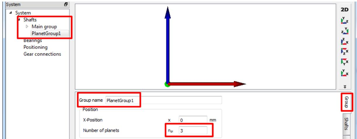
For the 'Main group' we add three shafts named 'Sun shaft1', 'Ring shaft' and 'Carrier shaft1'. For the PlanetGroup1 we add two shafts named 'Pin1' and 'Planet shaft1'.
