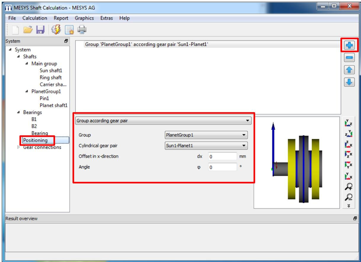
Add a constraint using the **+**-button on the right. Several options for positioning are available. Select 'Group according gear pair' and position 'PlanetGroup1 with pair 'Sun1-Planet1'. The angle could be changed, we just leave it to 0° for this example.
