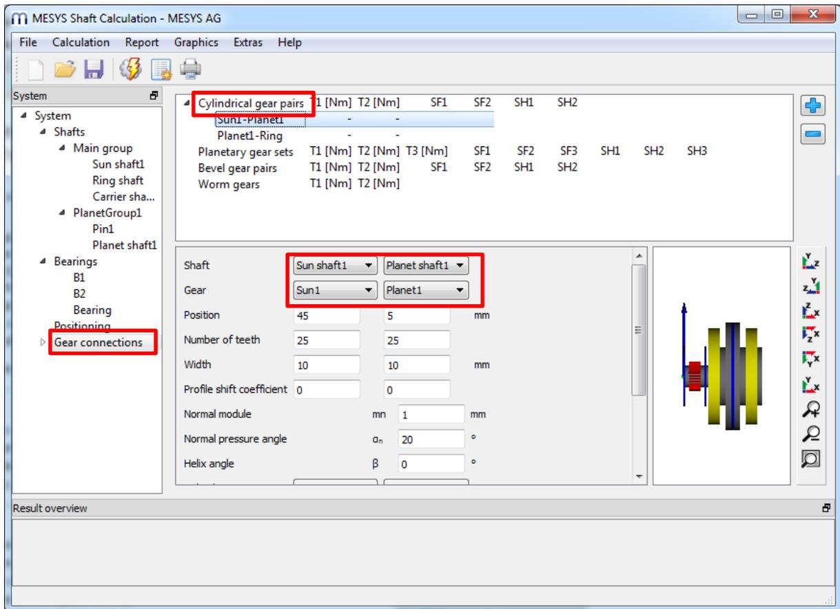
Now select the shafts and gears, which should be connected. Connect Sun1-Planet1 for the first pair, then add a second pair and connect Planet1-Ring. Circumferential backlash and gear mesh stiffness can be changed here. It is not needed to enter the center distance as it will be calculated later. The calculation program for the gear strength calculation can be selected if available.
