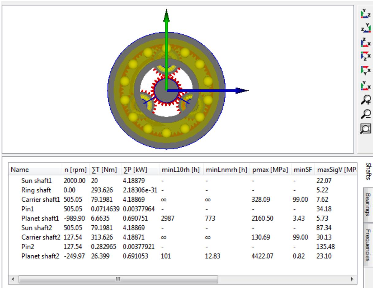
The output speed on Carrier2 is now 127.5 rpm, the output torque is 314Nm. The bearing life L10h is only 101h for planet shaft 2, which needs to be improved.
