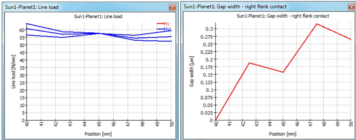
The line load shows the loading of all three contacts. The small difference is because of the weight of the shafts. The gap width shows the gap between the flank if the contact would be just on one point. So in this case a flank line correction of  $0.3\mu\text{m}$  could be made, but this small value can be ignored. Gear mesh stiffness, shaft and bearing stiffness have an influence to these diagrams. But also manufacturing errors and housing stiffness have an influence on the real gearbox.
