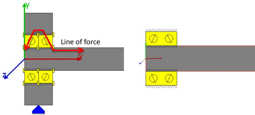
The support of the hollow shaft will be used to simulate the non-locating boundary conditions of the bearing set, since it will only support the hollow shaft radially and at the same time will also prevent the bearing set from torsion and tilting exactly as the housing would do:
