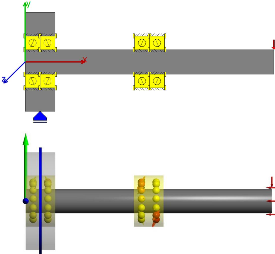
By connecting the outer rings of the bearings located at the middle of the shaft to the housing and setting all the flags corresponding to their supports conditions, the bearing set will behave as a fix support.
