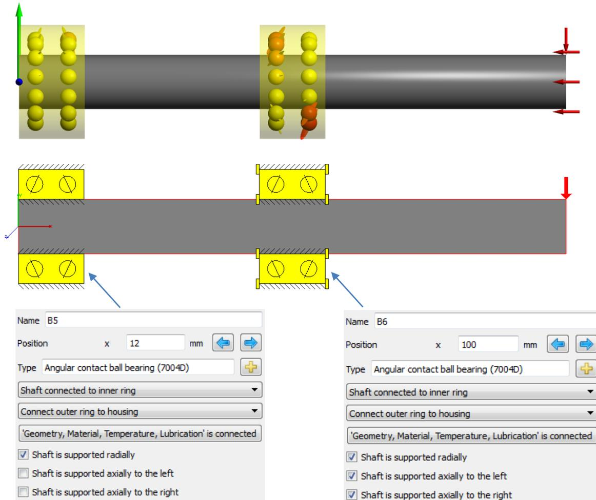
For both sets, groups of bearings are considered so that the corresponding bearings are located next to each other. More specifically, each pair of angular contact ball bearings will be arranged so that the distance of the bearing centers from the group origin is half of the bearing width, i.e.  $B/2 = \pm 6\text{mm}$ :
