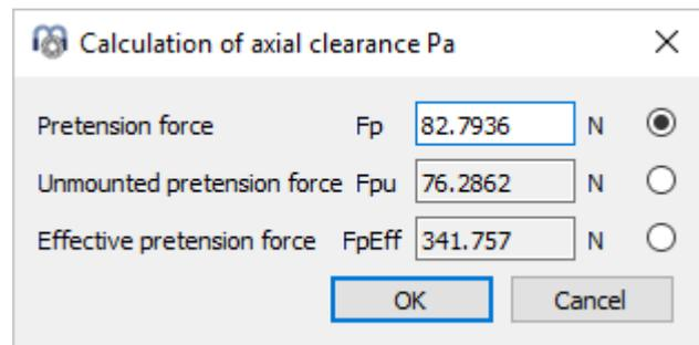
Dependent on the bearing type several options for the pretension force are available. The calculation with “Fp” is using nominal dimensions for the bearings, the calculation using “Fpu” is using nominal dimensions together with a radial elastic expansion without limit; this option can be used for the case of loading an unmounted bearing axially during manufacturing. The effective pretension force “FpEff” is calculated using the dimensions after fitting.
