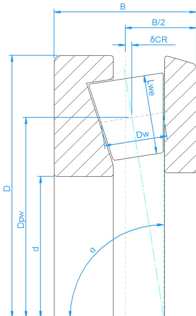
No tolerances are considered for axial tapered roller bearings.
