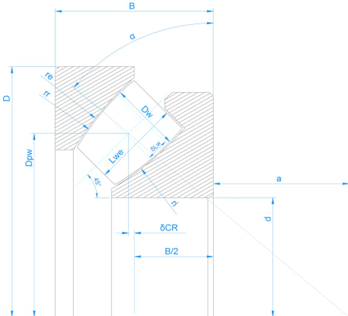
Radii of inner race and roller are defined by factors  $f_i$  and  $f_r$  like for the radial spherical roller bearings. They are defined as  $r_i = f_i \cdot (2 \cdot r_e)$  and  $r_r = f_r \cdot (2 \cdot r_e)$ . Default values are  $f_i = 0.5$  and  $f_r = 0.485$ . If the three radii  $r_i$ ,  $r_e$ ,  $r_r$  are entered using the -button behind  $f_i$ ,  $f_r$ , the factors  $f_i$ ,  $f_r$  and the pitch diameter  $D_{pw}$  are calculated.
