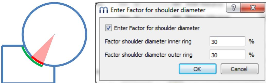
Instead of using an absolute value, the shoulder height can be defined using a percentage of ball diameters. A factor of 50% would be a shoulder up to the pitch diameter, so the factor should be between 10% and 40%. Using this factor allows to have default geometry on changing ball diameter or pitch diameter.
