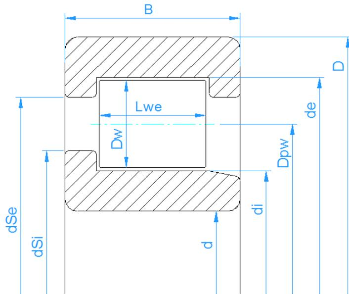
The roller profile is considered as defined by ISO/TS 16281 as default. If the extended calculation for pressure distribution is selected an input of profile for races and roller is possible using the  $\oplus$ -button behind the roller effective length. Several options are available including reading the profile from a file.
