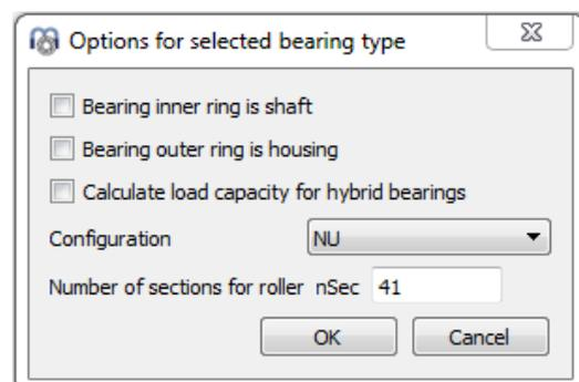
For NUP type the axial clearance is measured between left and right positions of the rings like for deep groove ball bearings. For directional bearings like NJ the axial clearance is between reference position and one side like for angular contact ball bearings or taper roller bearings.
