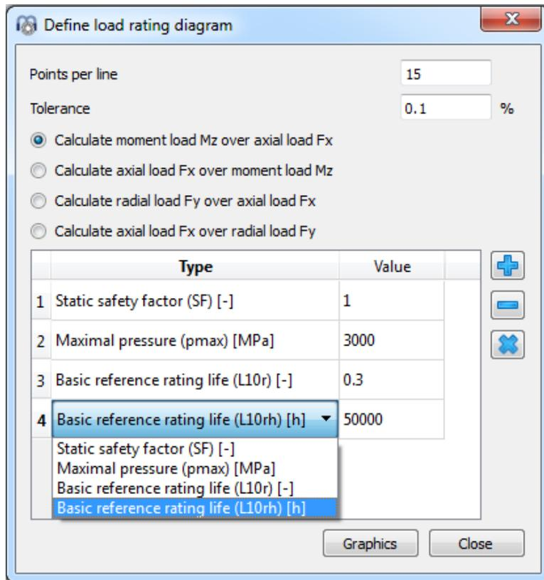
In the following picture it is shown a graphic example of the load rating diagram by which tilting moment (Mz) is compared against axial load (Fx) for a security factor of 1, Maximal pressure of 3000 Mpa, 300,000 cycles and 50000 h.
