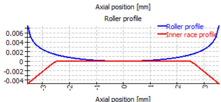
The unsymmetrical profile is used from left to right for most bearings. For taper roller bearings and axial spherical roller bearings the profiles is used from left to right if direction of contact angle is left. For contact angle to the right the profile is mirrored. So mounting conditions do not influence the profile.
