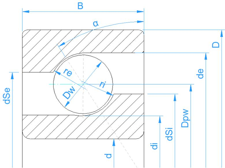
The direction of contact angle can be defined using the **+**-button behind the contact angle. Additionally, the input of direction of contact is available in the bearing type options.
