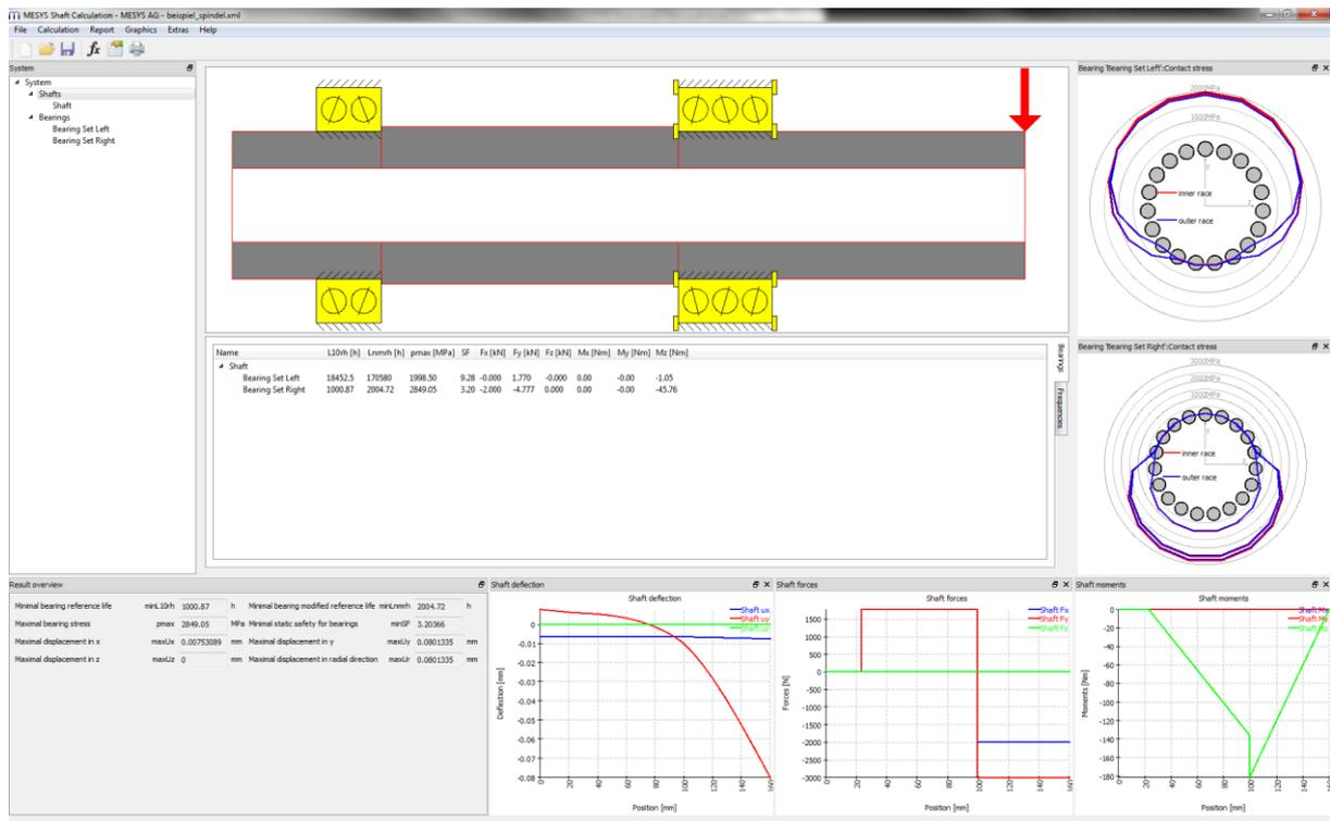
Shaft geometry can be defined using an arbitrary number of cylindrical and conical elements for inner and outer geometry. The geometry input is done using tables.
