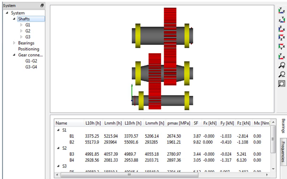
Gear pairs are considered as line load considering a mesh stiffness. The load distribution over the width of the gears provides a hint for necessary flank line corrections.
