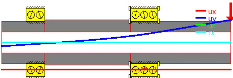
Additional masses can be defined for each shaft. The gyroscopic effect can be considered and a Campbell diagram is also provided in the software.
