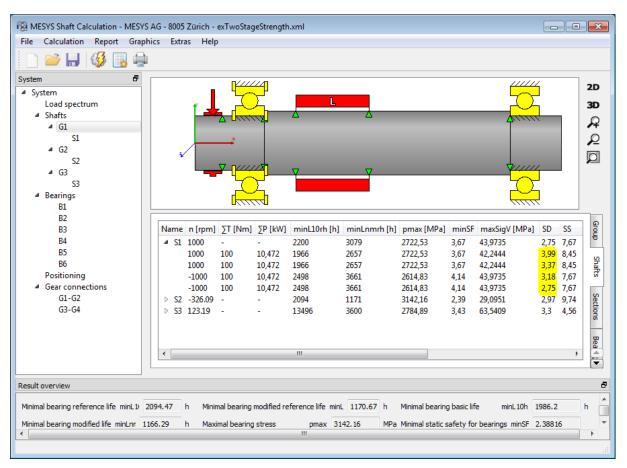
The strength verification according to DIN 743 will result in safety factors ranging from 2.75 to 3.99 with the four alternatives. The load case "Rotating direction Leftwards" with constant torsional torque is found to be critical. The results for the first three cross sections are as follows:
